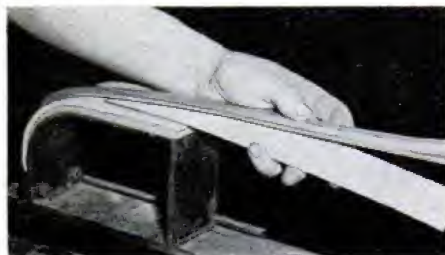
Above, the lemonwood lamination follows curve of the riser and is tapered to 1/64-in. thickness at the end. Below, professional bowmakers use a special bending jig of this type for bending recurve tips
